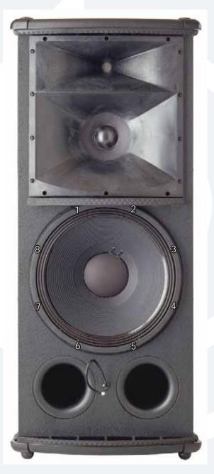
Eight screws and washers need to be removed from the woofer using the 4mm allen wrench.
